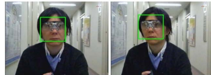
(a) Near infrared LED not lit (detection successful)
