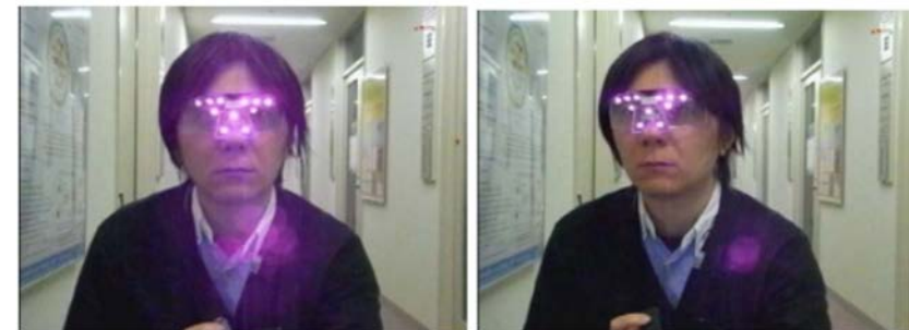
(b) Near infrared LED lit (detection failed)
